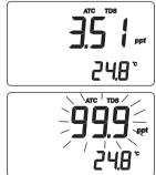
• If "lock" was pressed to freeze the LCD range and the reading is out of range, the full-scale value of the frozen range will blink on LCD.
