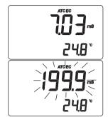
• If "lock" was pressed to freeze the LCD range and the reading is out of range, the full-scale value of the frozen range will blink.
