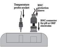
• The temperature probe is used in conjunction with the pH electrode to utilize the meter's ATC capability, but it can also be used independently to take temperature measurements. If the probe is disconnected, the temperature can be set manually using the arrow keys.
