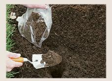
1. Collect samples of soil from the test area. (The soil should be taken from the same depth below the surface each time you test.) It is suggested to take at least two samples per test. The more samples, the more accurate the measurement will be. If you take more samples around your plant, then mix the samples. You will get a homogenous sample.
